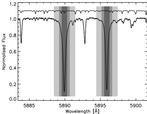
**Fig. 1.** Spectrum of HD209458 around the Na D doublet. The shaded areas indicate the narrow, medium, and wide passbands as used in our analysis. In all cases, the comparison bands are located directly adjacent to the central band, and have the same width. The upper line shows a synthetic telluric spectrum constructed from the line list of Lundstrom et al. (1991). Note that the telluric sodium absorption can show strong seasonal variability.
