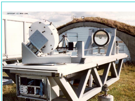
One of the 40cm diameter unit telescopes at the COAST array in Cambridge. The white rear face of the articulated siderostat mirror can be seen in the foreground. The collimated beam sent to the lab has a diameter of 25mm.
