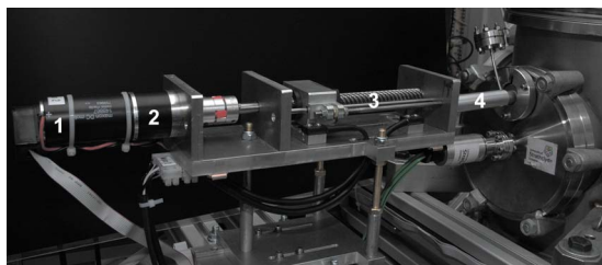
FIG. 4. (Color online) A close-up view of one of the two pistons in the new design. The labels indicate the dc motor (1), the gear box (2), the stainless-steel lead screw (3) with both the front and back switches, and finally, the vacuum feedthrough (4) with a protective cover.
