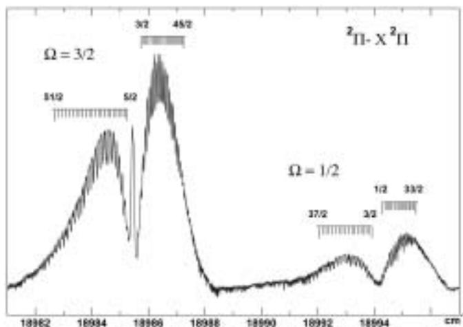
Fig. 3. The two rotationally resolved spin-orbit components of the origin band of the  $A^2\Pi - X^2\Pi$  electronic transition of  $C_6H$  measured by cavity ring down spectroscopy through a supersonic planar plasma. The intensity profile corresponds to a rotational temperature of about 15 K. (Reprinted from *J. Mol. Spectrosc.* 197, H. Linnartz *et al.*, Electronic ground and excited state spectroscopy of  $C_6H$  and  $C_6D$ , pp 1–11, Copyright (1999) with permission of Elsevier).
