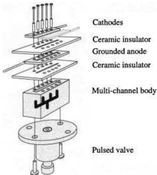
Fig. 1. A 3-D art view of the pulsed slit nozzle discharge system that is suitable to generate an intense supersonic planar plasma. Details on the construction are listed in the text. (Reprinted from Chem. Phys. 228, Birza *et al.*, Cw cavity ring down spectroscopy in a pulsed planar plasma expansion, pp. 119–224, Copyright (2002), with permission of Elsevier).
