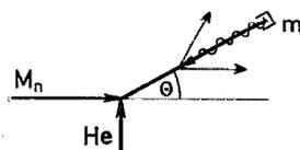
FIG. 1. Schematic view of the experimental setup. Both molecular beams, the cluster beam and the He beam, cross at an angle of 90° and can be rotated in such a way that the desired cluster size is scattered into the detector region where it interacts collinearly with the ir radiation of a homebuilt continuous wave CO<sub>2</sub> laser.
