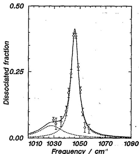
FIG. 7. The trimer dissociation spectrum for the 0.32%  $\text{CH}_3\text{NH}_2$  mixture in Ne measured at  $m = 63$  amu in the direct beam.
