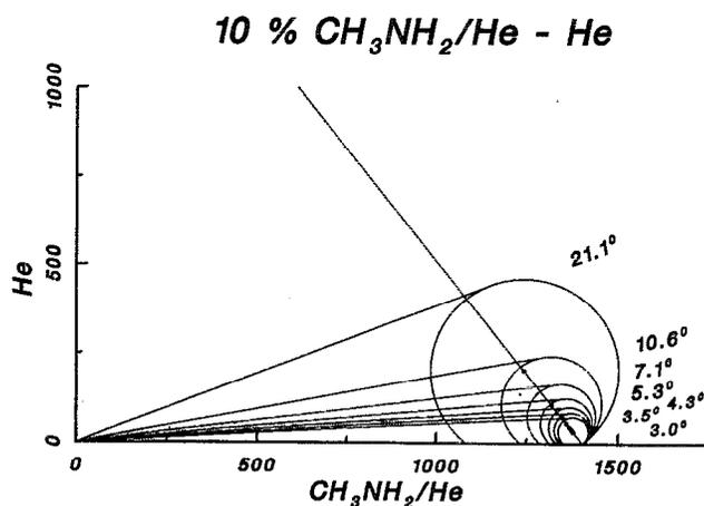
FIG. 2. The Newton diagram for the scattering of (CH<sub>3</sub>NH<sub>2</sub>)<sub>*n*</sub> clusters seeded in He by He. The positions of elastically scattered clusters are drawn for  $n = 1-7$  together with the listed limiting angles.
