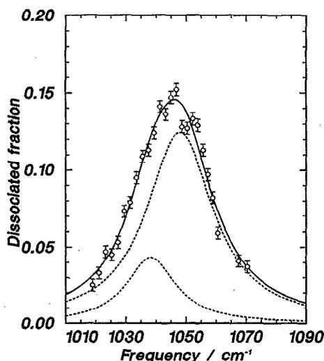
FIG. 5. The measured dimer dissociation spectrum for the 10%  $\text{CH}_3\text{NH}_2$  mixture in He at a scattering angle of  $8.5^\circ$ . The dashed lines are the results of a fit using the position of the resolved measurement of Fig. 8(A).
