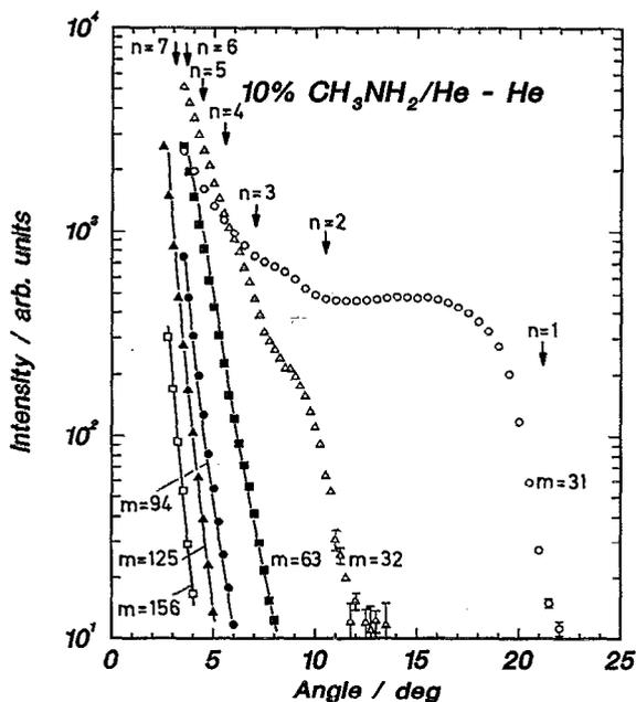
FIG. 4. The measured angular distribution of the scattered  $(\text{CH}_3\text{NH}_2)_n$  clusters seeded in He at different detection masses. The onset of intensity at the limiting angles is marked by arrows.
