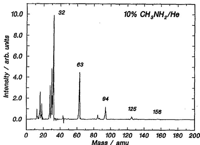
FIG. 3. The mass spectrum of a 10%  $\text{CH}_3\text{NH}_2/\text{He}$  mixture at a scattering angle of  $3^\circ$  which contains all clusters  $n < 8$ . The indicated mass peaks correspond to  $(\text{CH}_3\text{NH}_3)^+(\text{CH}_3\text{NH}_2)_{n-2}$  for  $n = 2$  to  $n = 6$ .
