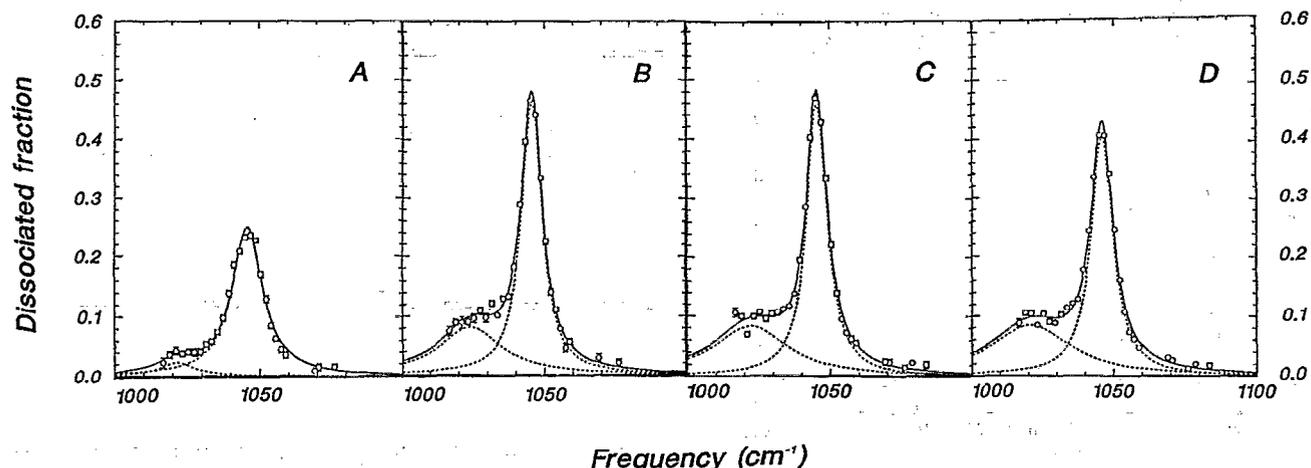
FIG. 6. The measured dissociation spectra for the clusters with  $n = 3$  to  $n = 6$  and the cluster composition of Table II. (A) is mainly the trimer spectrum at  $6^\circ$  ( $m = 63$  amu), (B) the tetramer spectrum at  $5^\circ$  ( $m = 94$  amu), (C) the pentamer spectrum at  $4^\circ$  ( $m = 125$  amu), and (D) the hexamer spectrum at  $3^\circ$  ( $m = 156$  amu).
