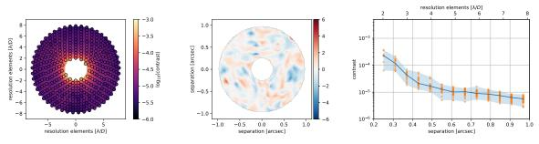
Figure 5. (left) The calibrated contrast floor for an SNR=5 signal in the example gvAPP-180 data as a function of position in the final derotated focal plane. (middle) The SNR measured at each point with the optimal hyperparameters for that focal plane location (without any injected signal). (right) The calibrated contrast curve as a function of separation, with the shaded region encompassing the variation with position angle.
