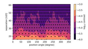
Figure 4. The calibrated contrast floor for an SNR=5 signal as a function of position angle and separation, shown in unwrapped rectilinear coordinates after interpolation and contour-calculation. The focal plane sampling (black points, also shown in Figure 5) gets finer in PA as separation increases. The final contrast surface exhibits clear structure with two maxima in contrast as a function of PA.
