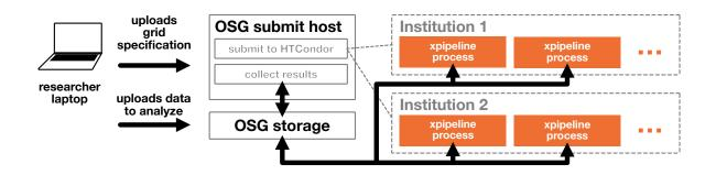
Figure 6. Illustration of the operation of XPipeline on the Open Science Grid. Rather than farming the tasks out through a central coordinator process, the task arguments are determined before submission and supplied to the xpipeline process through HTCondor. This uses the grid framework in xpipeline, but does not necessarily leverage Ray.
