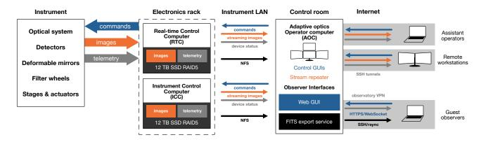
Figure 1. Command and data flow within MagAO-X, organized with the instrument hardware on the left and control computers on the right. The adaptive optics control computer (AOC) runs control GUIs locally, but also serves as the home for guest observer services like reduced-frame-rate image streams, web GUIs, and the service that produces science-ready FITS files for observers.
