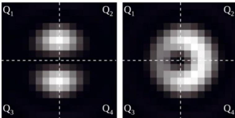
Figure 4. Quadrant analysis of the coronagraphic image in the case of a non obstructed pupil (left) for the four quadrant phase phase mask and (right) for the vortex phase mask. The tip-tilt amplitude is  $0.2 \lambda/D$  and the image width is  $4 \lambda/D$ .
