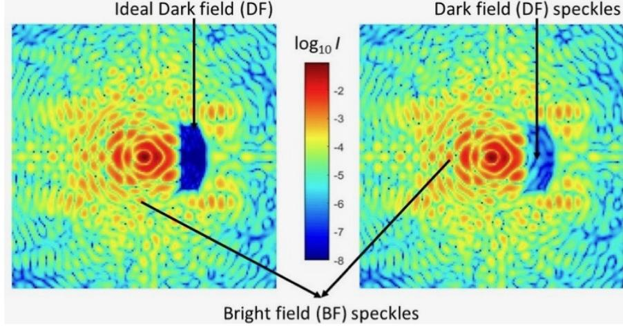
Figure 2. (Left) Spatial LDFC:  $3.5 \lambda/D \times 8.5 \lambda/D$  dark hole/dark field (DF) created in numerical simulation using conventional electric field conjugation (EFC). (Right) Wavefront aberrations produce speckles in the bright field (BF) and the DF which degrade the DF. The change in intensity between the aberrated BF (Right) and the ideal BF (Left) is used to measure and cancel the speckles in the DF.
