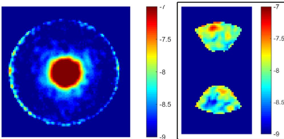
Figure 8. Laboratory results from WFIRST CGI testing at JPL, using pairwise probing for wavefront estimation. Both are shown on the same base-10-log contrast scale. *Left.* Best narrow-field-of-view result with an HLC coronagraph ( $1.6 \times 10^{-9}$  contrast  $3 - 9\lambda/D$ , 10%) *Right.* Best spectroscopy-mode result with an SPC coronagraph ( $1.1 \times 10^{-8}$  contrast  $3 - 9\lambda/D$ , 18%)
