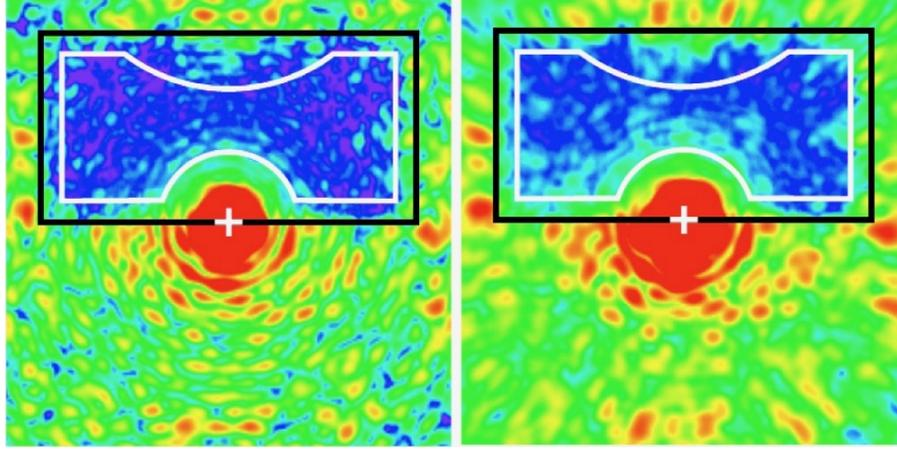
Figure 6. SCC Laboratory results. (Left) Half dark hole ( $13 \times 27 \lambda/D$ ) obtained in monochromatic (650nm) and (Right) broadband (12,5% bandwidth in visible) light using the SCC as a focal plane wavefront sensor. The bottom of the dark hole (blue and purple colors) is  $10^{-8}$  contrast [47](#).
