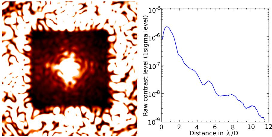
Figure 7. SCC Laboratory results. (Left) Full dark hole ( $17 \times 17 \lambda/D$ ) obtained in monochromatic light (785nm) using the SCC as a focal plane wavefront sensor and two deformable mirrors. No CDI is applied. (Right) Normalized azimuthal standard deviation associated to the image [50](#).
