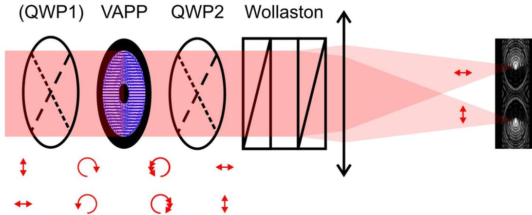
Figure 1. Working principle of the vector-APP.
