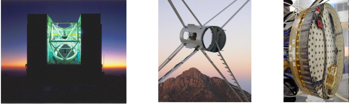
Figure 2. The MMT AO System. The successive pictures show the 6.5m MMTO telescope, the deformable secondary mirror in the telescope hub, and a detail of the secondary mirror during assembly in the optics laboratory showing the location of the 336 mirror actuators.
