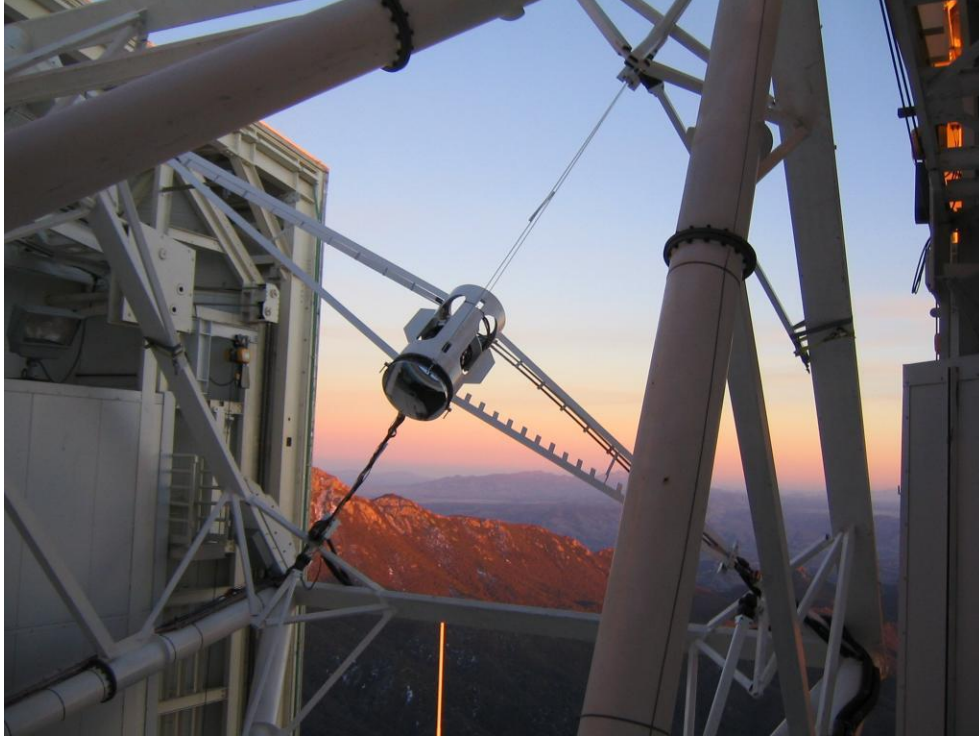
Figure 1. The adaptive secondary installed at the MMT telescope. In the foreground the telescope structure, in the background the Arizona desert south of Tucson. This photo was taken during the Jan-Feb 2004 run.
