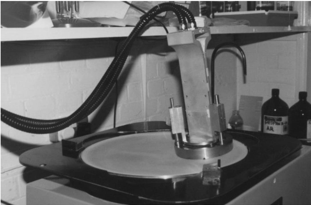
**Figure 5-22** *The curved fibre slit on the spherical polishing plate.*
