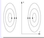
separate magnetic field into azimuthal (toroidal) and poloidal (radial and axial) components
