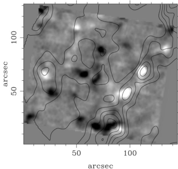
Magnetogram of quiet Sun close to disk center with contour lines showing 2-cm radio emission intensity as observed with VLA
