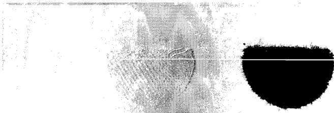
Figure 5: Negative contrast display of cross talk among four quadrants of a Rockwell Scientific Company HyViSI-1024 camera. The range shown is 0 to 5% of the maximum illumination level. This image has been dark-corrected. Large-scale shading is scattered light.
