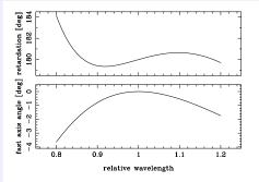
Theoretical variation of retardation and fast axis orientation as a function of relative wavelength for a Pancharatnam achromatic half-wave plate
