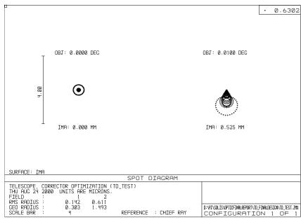
The telescope is a quasi RC system and has to work with the corrector. The above drawing show there is a non-spherical aberration position on the axis which can be used for the primary and secondary mirror combination testing.
