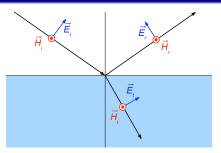
ratios of reflected and transmitted to incident wave amplitudes
