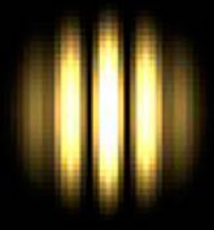
Fringe pattern seen by interferometer
