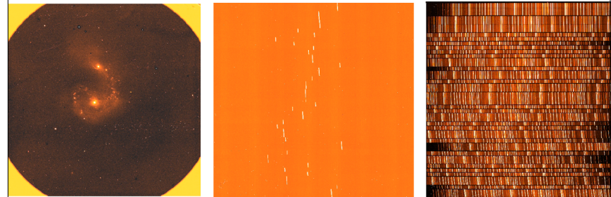
Figure 7. On the left is the layout of the MOSFIRE field on the sky with a 58s J-band image of The Antennae galaxies. The middle image is of a slit mask and the right image is the night sky emission with this mask in H-band.
