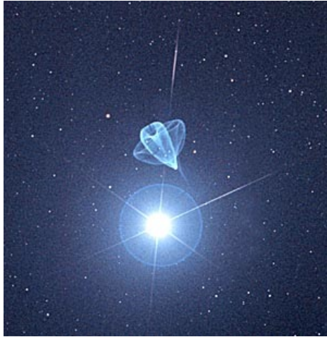
Internal reflections from a Schmidt camera
