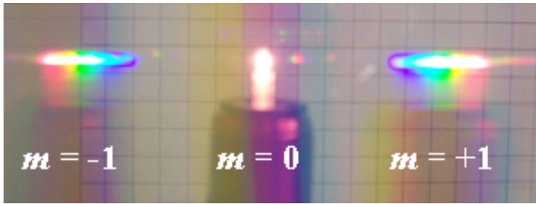
A light bulb seen through a transmissive grating, showing three diffracted orders. m = 0 corresponds to direct transmission; colors with increasing wavelengths (from blue to red) are diffracted at increasing angles. Source: Wikipedia
