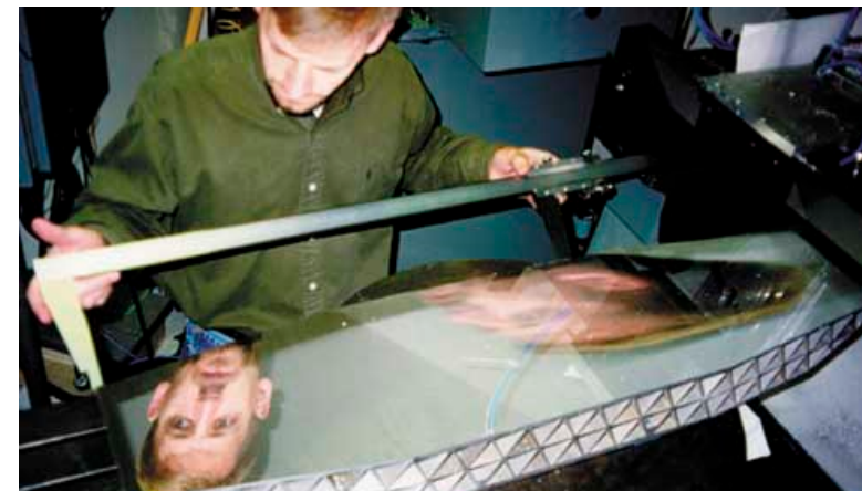
The ruled echelle grating of the SOFIA Facility Spectrometer ARIES. Two images of the engineer are seen reflected from the facets of the grooves that are at angles of 90 degrees from each other.
