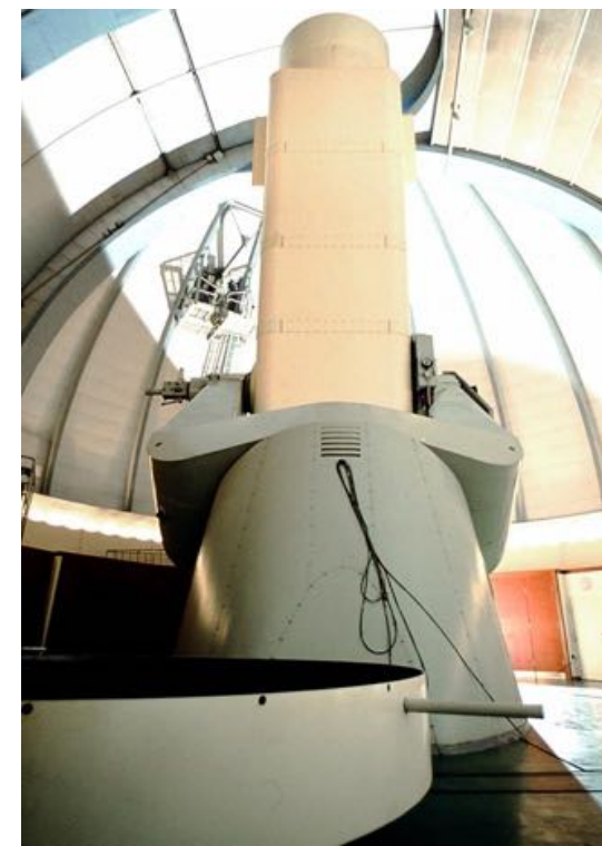
Two meter Alfred-Jensch-Telescope in Tautenburg, the largest Schmidt camera in the world.
