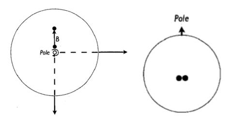
1. Consider a source located at the pole, and a simple two telescope interferometer (see left figure). Imagine you are the source, looking down at the Earth. What u, v-points do you gather as the Earth rotates?
