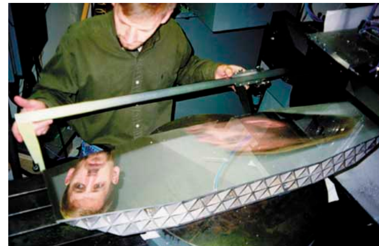
The ruled echelle grating of the SOFIA Facility Spectrometer AIREs. Two images of the engineer are seen reflected from the facets of the grooves that are at angles of 90 degrees from each other.
