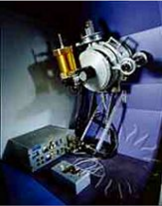
The "single pixel" Ge:Ga bolometer invented in 1961 by Frank Low
