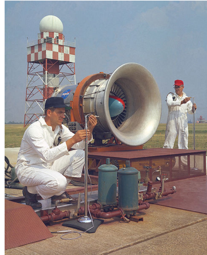
NASA researchers at Glenn Research Center conducting tests on aircraft engine noise in 1967
