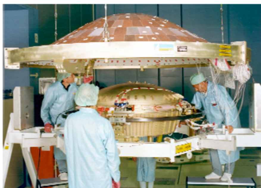
Figure 7: The Huygens probe during assembly
