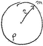
force on the test mass  $m$ :  $F = \frac{GM_m}{r^2} = \frac{4\pi G}{3} \rho m r^2$  (with  $M = \frac{4\pi}{3} \rho r^3$ )
