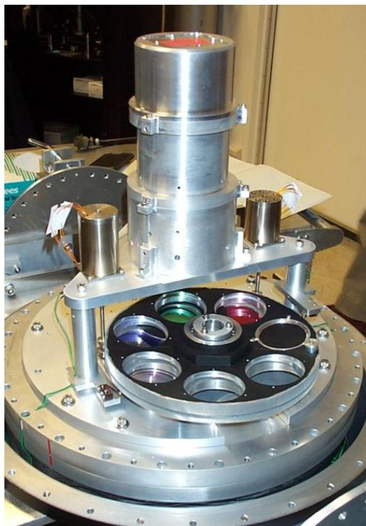
**Figure 3.** The WIRC dewar opened in the lab. The 4-lens collimating section can be seen in its lens barrel assembly. The two filter wheels straddling the Lyot stop can also be seen just above the cold plate.
