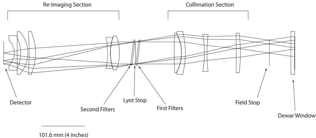
**Figure 1.** A schematic of the WIRC optical train from the dewar window (right side) to the detector (left side). Three beams are also shown: the on-axis beam and two at the edge of the field.
