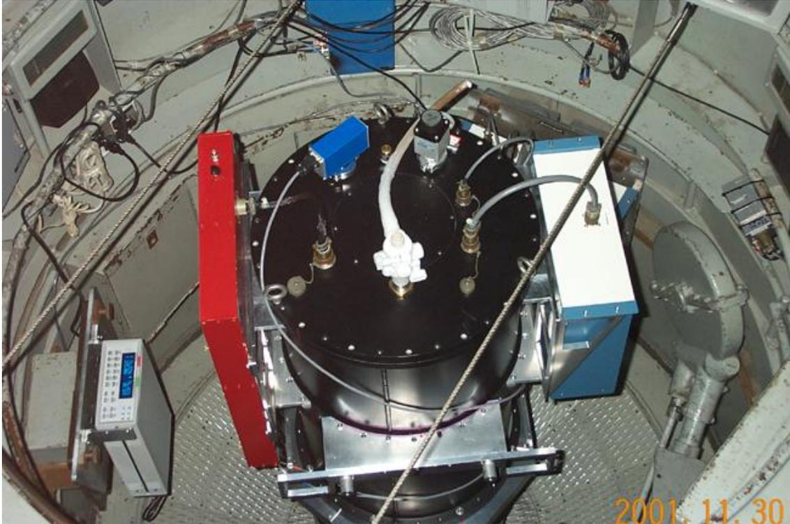
**Figure 4.** WIRC mounted at the prime focus of the 200-inch telescope for first light.
