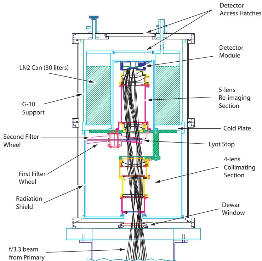
**Figure 2.** A schematic of the WIRC dewar and optics.
