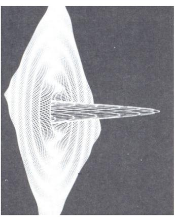
Remember: the **Rayleigh criterion** states that two sources can be resolved if the peak of the second source is no closer than the 1<sup>st</sup> dark Airy ring of the first source.
