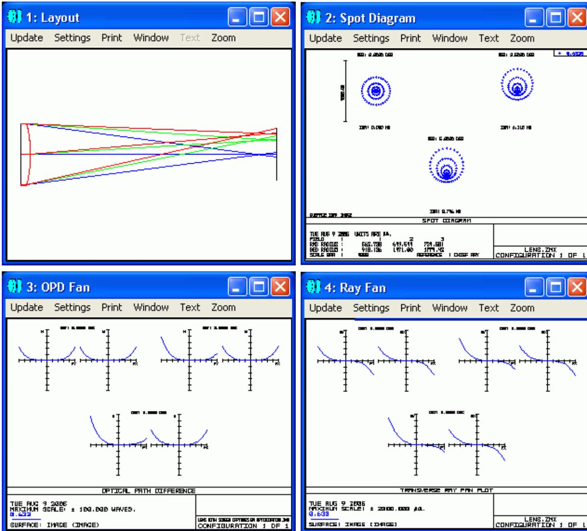
From evaluation of the four plots above, it is obvious that the singlet design has a significant number of aberrations, including but not limited to spherical, coma, distortion, defocus, field curvature, and astigmatism. In addition, the geometrical and RMS radii (as is reported at the bottom of the Spot Diagram) at the maximum field are roughly 734.581 and 1774.42 $\mu\text{m}$ , respectively.
