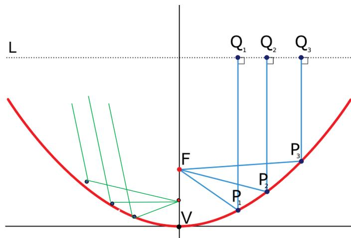
→ FOV is limited by aberrations: the bigger the mirror the bigger the difference [parabola - sphere] near the edge → bigger telescopes have smaller FOVs ( $\sim < 1$  deg).
