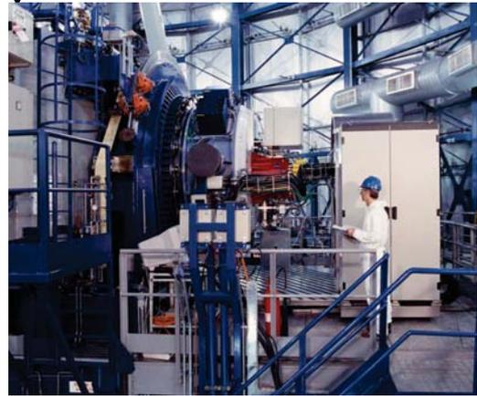
**Nasmyth** - ideal for heavy instruments to put on a stable platform, but field rotates
