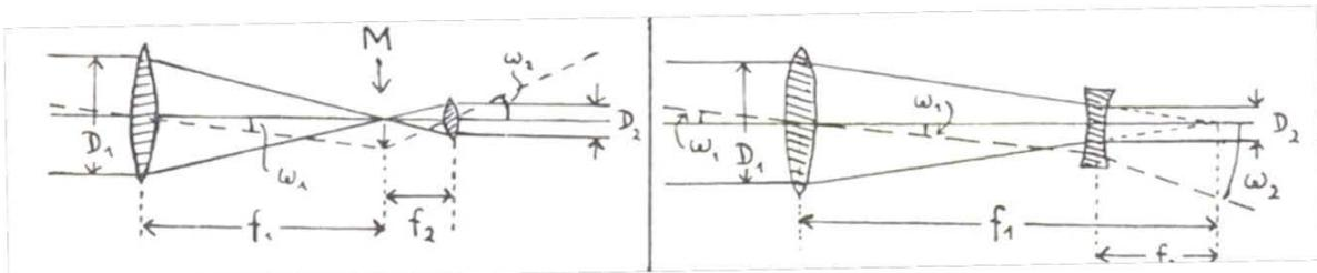
Magnification:  $V = \frac{f_1}{f_2} = \frac{D_1}{D_2} = \frac{\omega_2}{\omega_1}$
