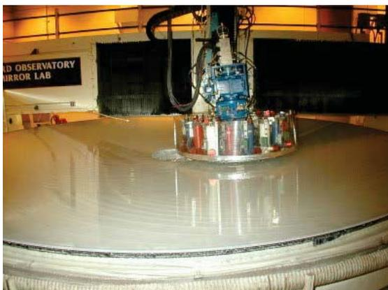
Polishing a 6.5-m mirror on the Large Optical Generator (LOG) using the stressed-lap polishing tool. The lap changes shape dynamically as it moves radially from center-to-edge of the mirror to produce a paraboloid. Our 6.5-m mirrors are typically figured to a focal ratio of  $f/1.25$  with a finished precision of  $\pm 15\text{-}20$  nanometers.
