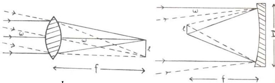
Scale:  $\tan \omega = \frac{l}{f}$  and for small  $\omega$ :  $l \approx 0.0175 \omega f$
