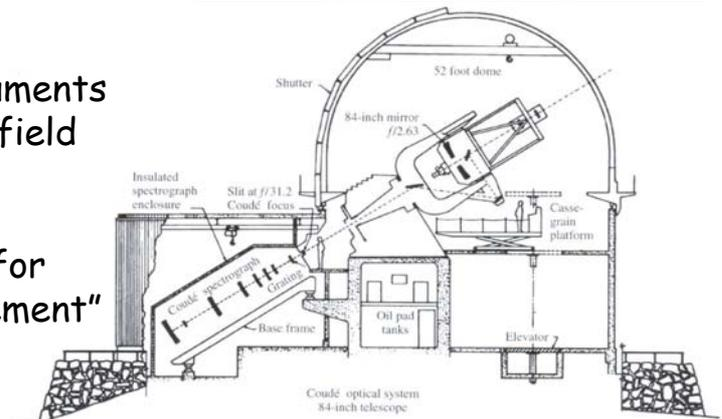
Fig.3.13. The coude system of the Kitt Peak 2.1 m reflector. (Drawing National Optical Astronomy Observatories, Kitt Peak National Observatory)
