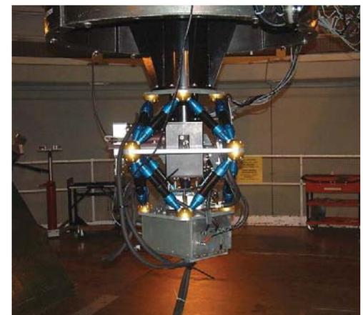
**Prime focus** - wide field, fast beam but difficult to access and not suitable for heavy instruments
