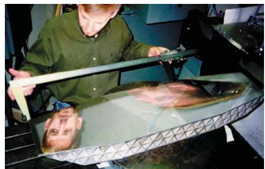
The ruled echelle grating of the SOFIA Facility Spectrometer ARIES. Two images of the engineer are seen reflected from the facets of the grooves that are at angles of 90 degrees from each other.
