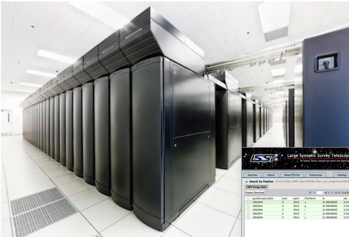
*A petascale supercomputing system at the **LSST Archive** (at NCSA) will process the raw data, generating reduced image products, time-domain alerts, and catalogs.*
