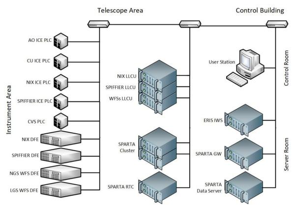
Figure 2: Conceptual architecture of ERIS control network.
