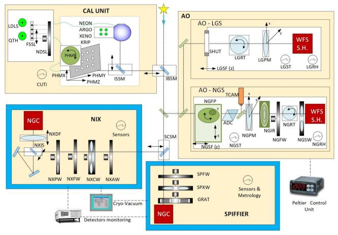
Figure 1: Conceptual view of ERIS Instrument functions.
