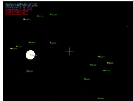
Figure 5. Example of the star Tracker image analysis results. Stars in the frame are identified by their catalog number. The azimuth and elevation of the telescope is also calculated from the image.
