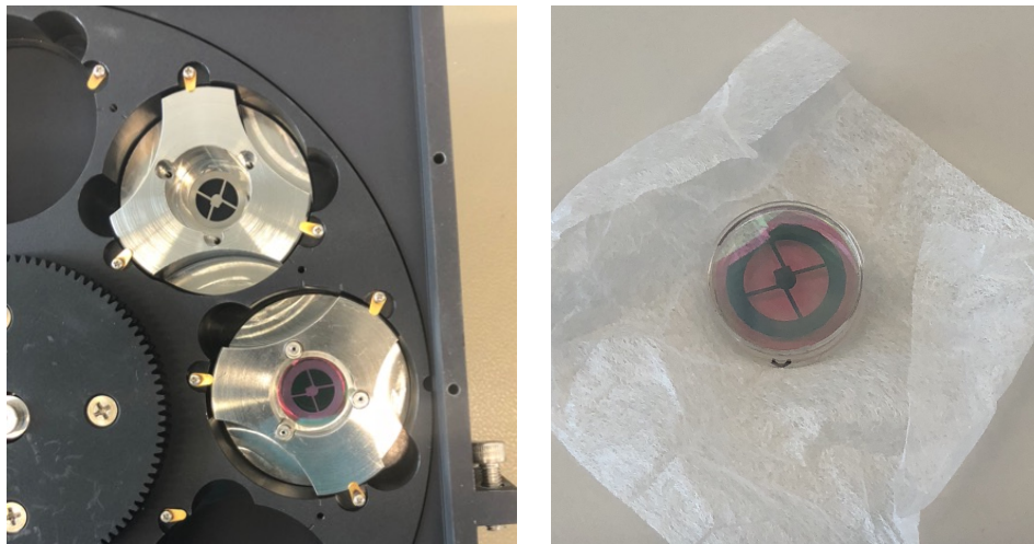
Figure 4. Left: image of the VLT pupil mask (top) and the ERIS gvAPP (bottom) installed in the first filter wheel of the second pupil plane in the ETH Zurich cryogenic near-infrared test bench. Right: close up view of the gvAPP coronagraph. The VLT pupil mask is identical to the pupil mask included in the gvAPP and is used to produce a nominal PSF to compare with the PSF of the gvAPP. For reference, the VLT pupil mask is 11.3 mm (0.45 inches) in diameter.
