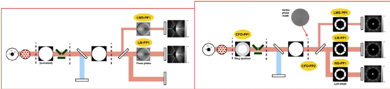
**Figure 7** Simplified diagrams of the optical system, showing the locations of the coronagraphic masks at the various pupil planes (PP) and focal planes (FP) within METIS. *Left*: The apodized phase plates (APP). *Right*: The ring-apodized vortex coronagraph (RAVC).
