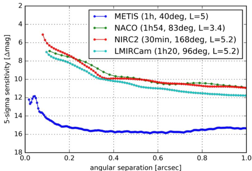
**Figure 8** Simulated contrast curve for the METIS ring-apodized vortex coronagraph at L band after 1 hour of on-sky integration, assuming 40 degrees of sky rotation and no non-common path aberrations between the wavefront sensor camera and the science camera in the focal plane. Comparison curves from current 8 m class telescopes are shown as blue, green and red curves.
