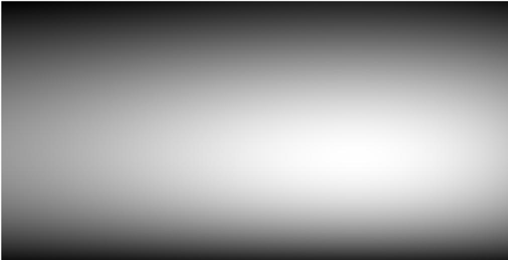
**Figure 6-13** *A scattered light image.* This image is a fit to the scattered light in a twilight sky exposure from the SPIRAL spectrograph. The values range from 246 DN in the middle to 26 DN at the edges. The optical axis of the spectrograph passes through the middle right of the frame.
