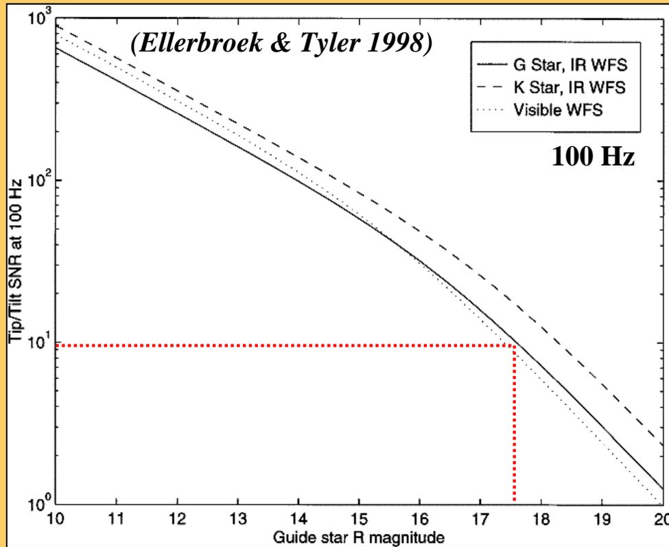
At 100 Hz one can achieve sufficient S/N with sources as faint as 17.7 mag
