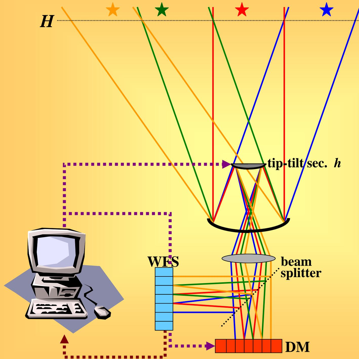
→ The deformable mirror (DM) must be conjugated to the height  $H$
