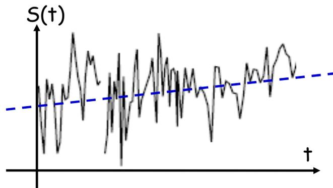
**Gaussian noise** - noise with a Gaussian amplitude distribution (normal distribution), i.e., the noise values are Gaussian-distributed\*.
