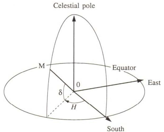
Fig. 8.3. The hour system of coordinates
