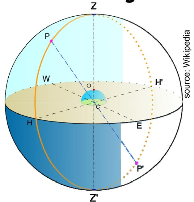
An **hour angle** is the angle described by the earth rotation in one hour
