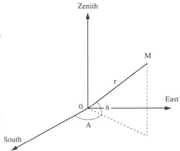
Fig. 8.2. Definition of the horizontal reference system
