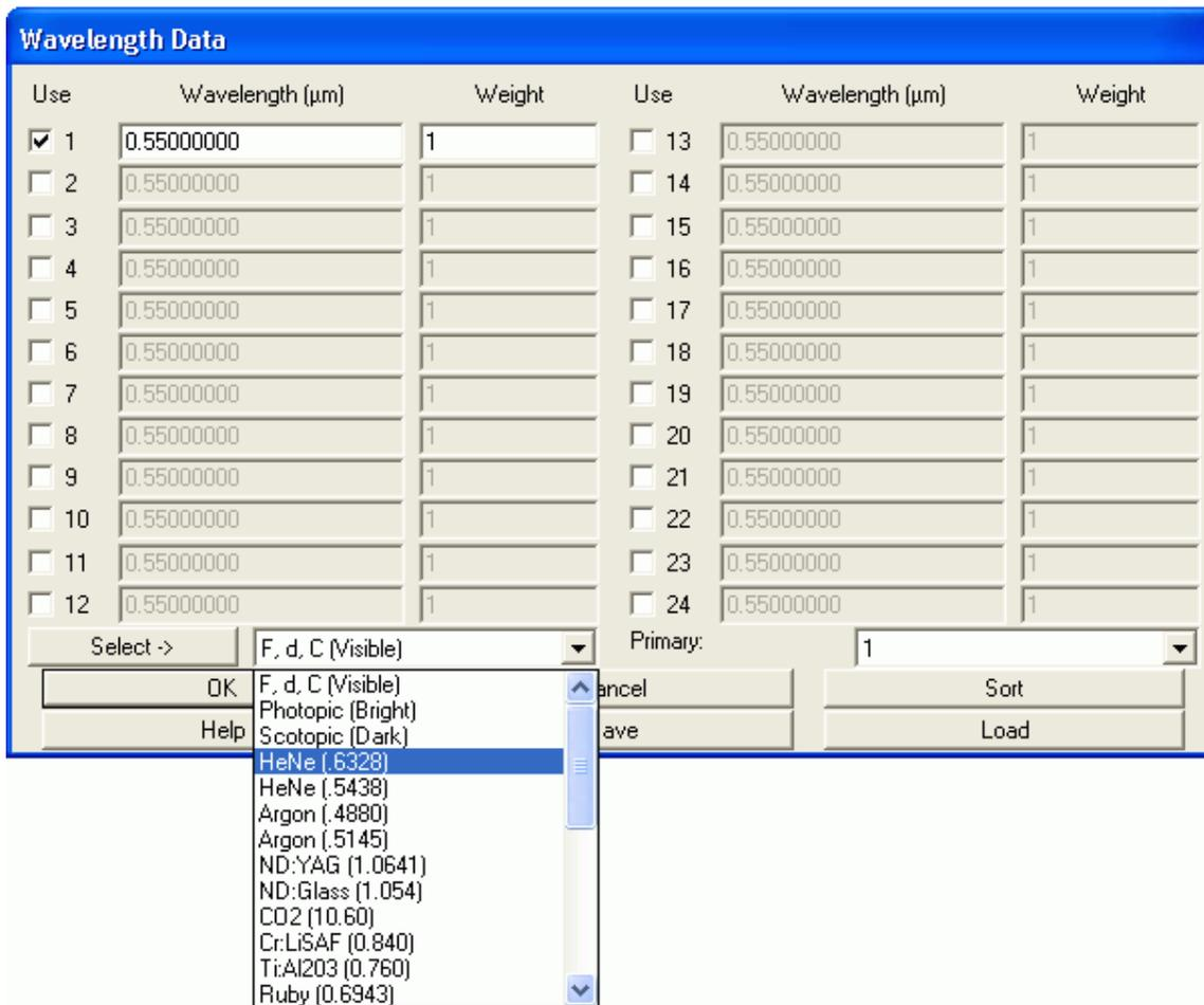
F, d, C (Visible) is the first option by default. However, choose the current design wavelength by first selecting *HeNe (.6328)* from the pull-down menu, and then pressing the “Select ->” button which is next to the pull-down menu. ZEMAX will automatically place this wavelength into the first entry:
