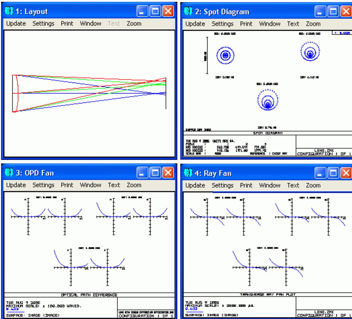
From evaluation of the four plots above, it is obvious that the singlet design has a significant number of aberrations, including but not limited to spherical, coma, distortion, defocus, field curvature, and astigmatism. In addition, the geometrical and RMS radii (as is reported at the bottom of the Spot Diagram) at the maximum field are roughly 734.581 and 1774.42 $\mu$ m, respectively.
