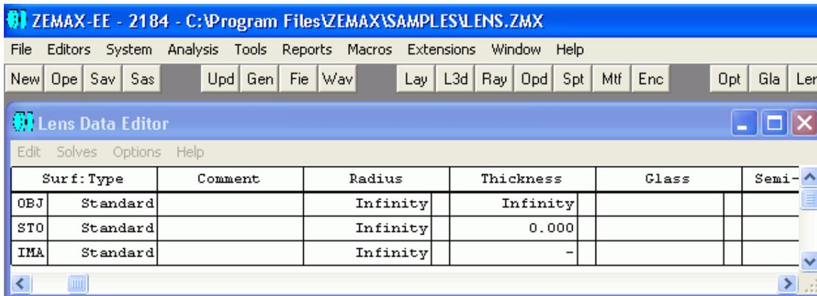
Each row within the LDE represents a single surface. In sequential ZEMAX, each optical system begins at the object (OBJ) and ends at the image (IMA). In addition to the object and image planes, one of the surfaces must be defined as the aperture stop (STO).
