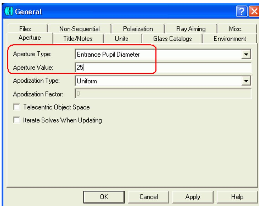
The Aperture Value is considered to be in *Lens Units*. The lens units define the units of measure for dimensions in most of the spreadsheet editors in ZEMAX. These dimensions apply to data such as radii, thicknesses, EPDs, and most other parameters in ZEMAX. It is very important that the system units be defined prior to starting the design. Always check to verify that the system lens units are what you expect them to be!
