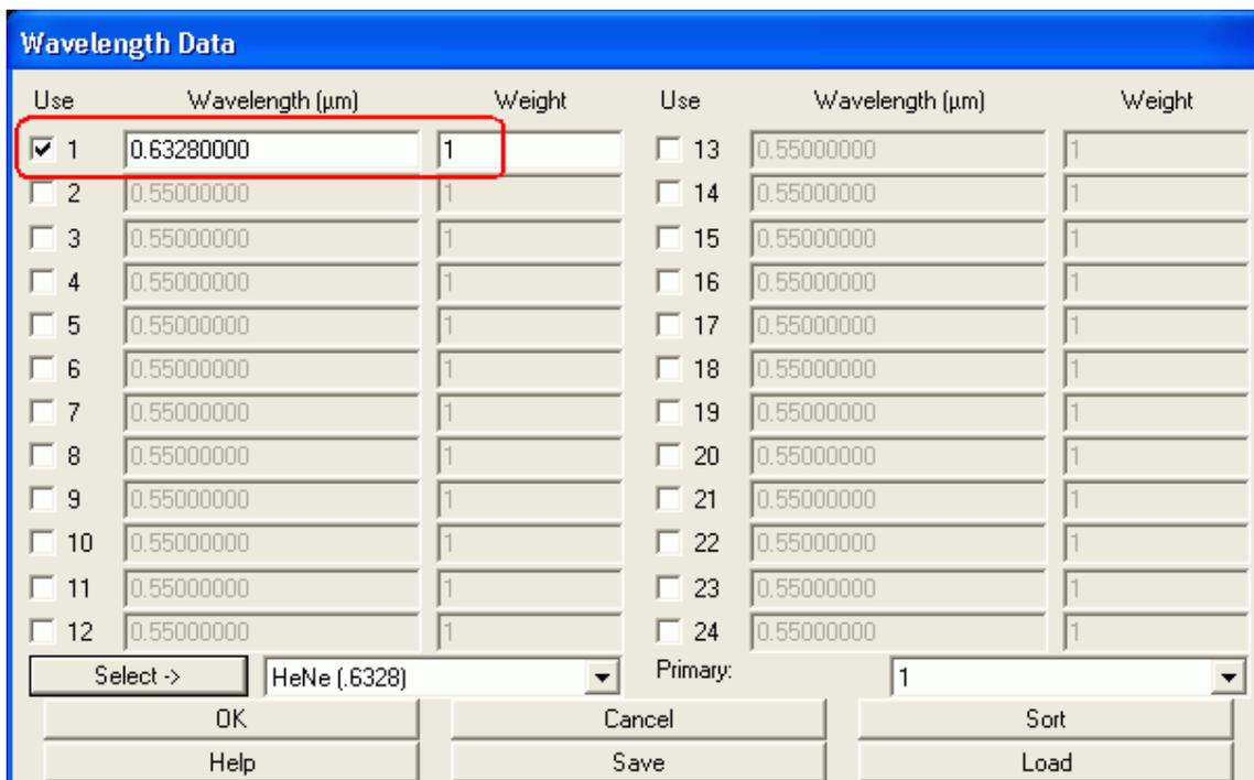
*Note that wavelengths in ZEMAX are always entered in microns, regardless of the system lens units!*
