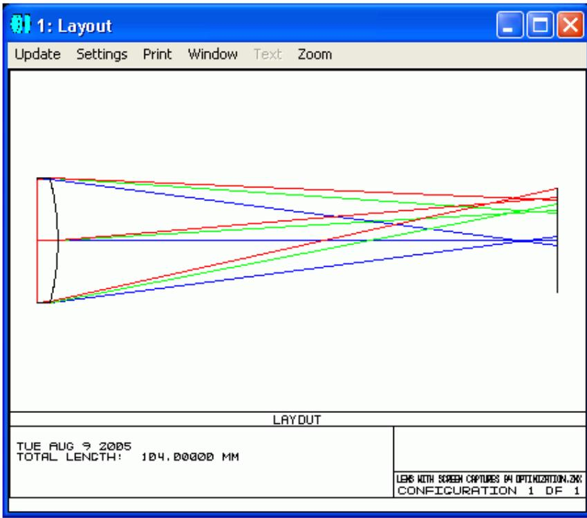
Even prior to optimization, we can use a tool within ZEMAX to better position the current image plane location. The tool is known as the *Quick Focus* tool. Quick Focus is a feature in ZEMAX which adjusts the thickness of the surface prior to the image plane to minimize the RMS aberrations.
