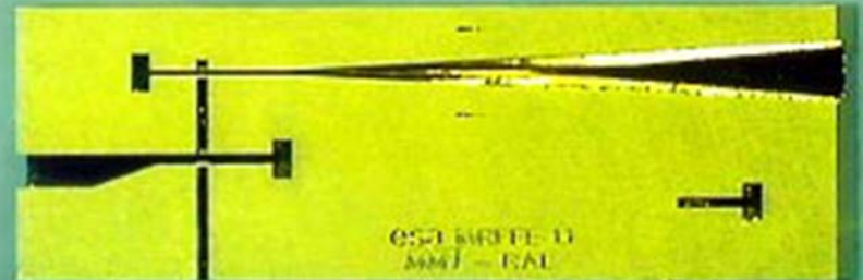
560 GHz micro-machined sub-harmonic mixer
