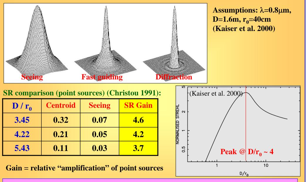
Gain ~ 4 means: same S/N as from a seeing limited telescope  $\frac{4 \times bigger}{D}$  in diameter since S/N  $\propto$  D/source (BLIP)
