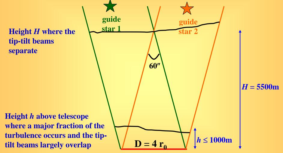
Now "assemble" a large FOV from many adjacent tip-tilt beams. The tilt-isoplanatic patch (here 60" across) replaces the turbulence cell ( $r_0$ ) in conventional AO "thinking". For correction use a system similar to a conventional AO system.
