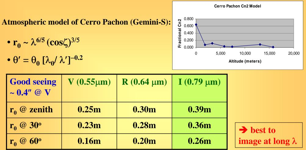
Mean  $r_0 \sim 0.35m$  @ I-band  $\rightarrow$  telescope diameter  $\sim 4r_0 = 1.4 m$
