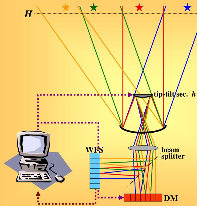
→ The deformable mirror (DM) must be conjugated to the height H
