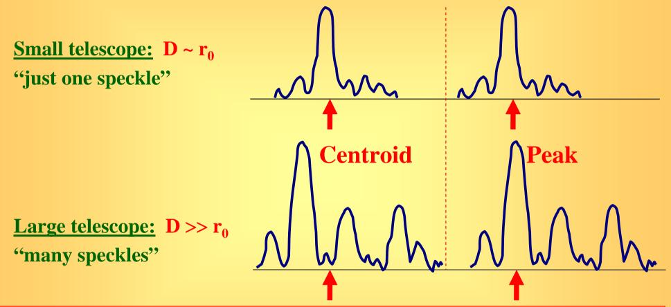
• **Centroid tracking requires:** quad-cell detector (only possible option here!)
